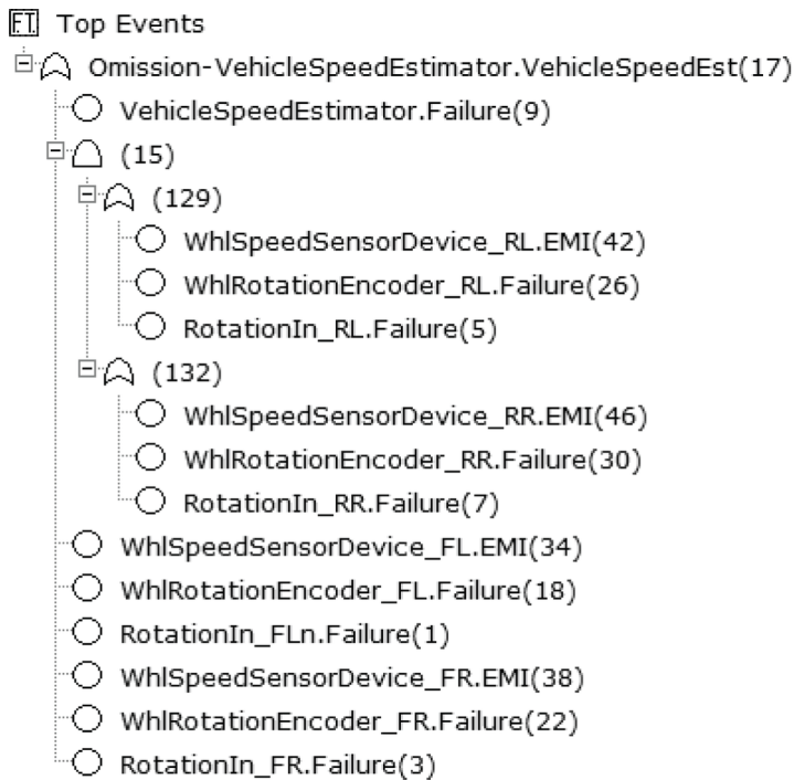
Figure 18. The HiP-HOPS synthesized fault trees for omission of vehicle speed estimator
