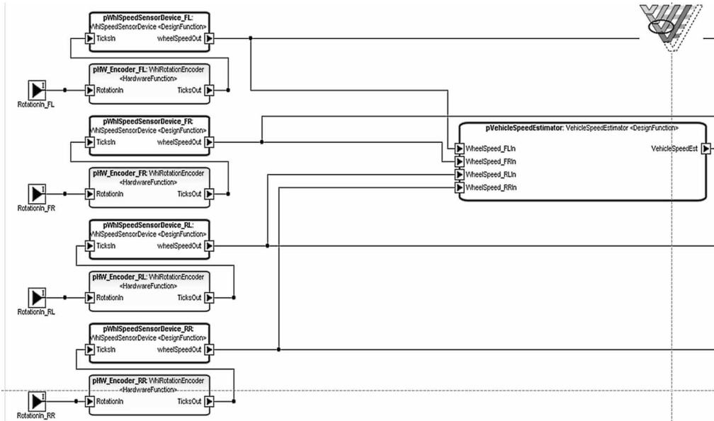
Figure 8. Hardware architecture of the regenerative braking system
