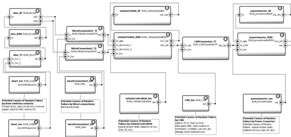
Figure 16. A state-machine based error logic description
