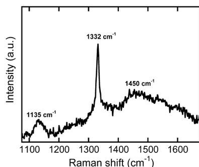
FIGURE 10. Raman spectra of the diamond film (ND-30/PDDAC) on a silicon substrate after 60 min of CVD plasma growth.
