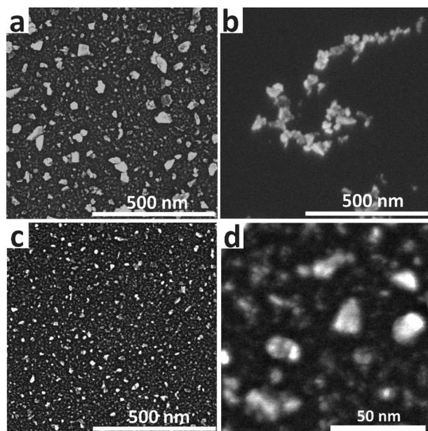
**FIGURE 2.** SEM pictures of a silicon substrate after 15 min of immersion in ND-50 solution: (a) with PDDAC polymer coating; (b) without PDDAC coating; (c, d) a silicon substrate coated with PDDAC after 15 min of immersion in ND-15 solution.
