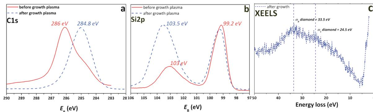
FIGURE 9. XPS analysis giving (a) C 1s and (b) Si 2p core level spectra (normalized) and (c) XEELS spectra (C–C  $sp^3$  peak as the energy loss origin) of diamond nanoparticles (ND-50) deposited on PDDAC-coated Si substrate before (solid line) and after (dashed line) 10 min of CVD plasma growth (see the Experimental Section).
