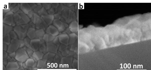
FIGURE 7. SEM images giving (a) a top view of the diamond thin film (ND-30/PDDAC) after 45 min of CVD plasma growth and (b) a cross-section view of two ND-30/PDDAC layers after 25 min of CVD plasma growth.
