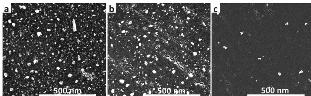
FIGURE 3. SEM pictures of diamond nanoparticles deposited on a PDDAC-coated Cr substrate using (a) ND-30 solution over 1 min, (b) ND-30 solution over 5 s, and (c) ND-30 solution diluted  $c/10$  over 5 s.
