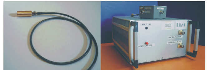
Fig 3. View of the fiber-coupled scintillator (BGO) for the detection of ambient scattered radiation (left) and associated discriminating unit and logic gate (on top) developed by the CEA LIST (right).
