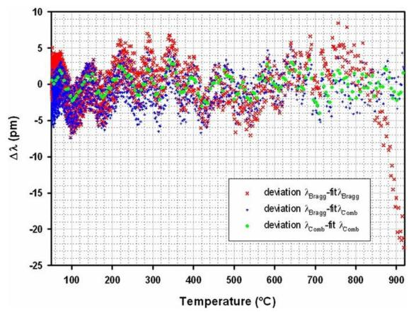
**Figure 7.** Deviations between the experimental Bragg wavelengths with regard to a fifth-order polynomial fitting processed on averaged (blue point, subset averaged every 5 °C) and non-averaged (red point) data. The green points stand for the error between the averaged data and the polynomial fit computed thereon.
