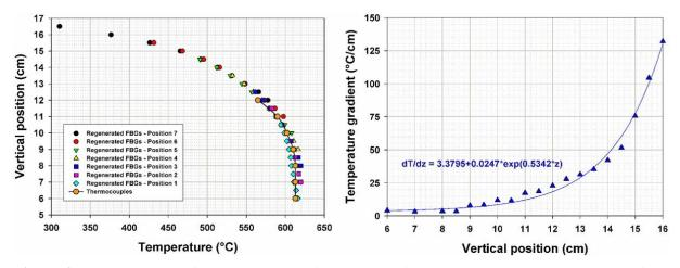
**Figure 8.** Temperature profile and gradient of the tubular furnace reconstructed by an array of ten multiplexed regenerated FBGs.
