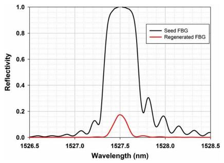
**Figure 4.** Spectrum of a seed FBG and that of the corresponding regenerated FBG (both spectra acquired at room temperature).
