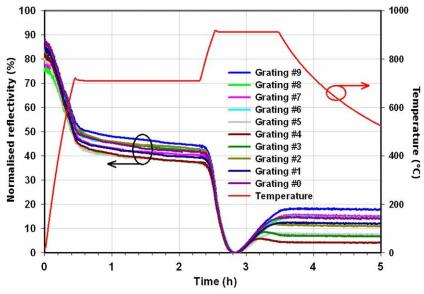
**Figure 5.** Evolution of the reflection signal from the ten multiplexed seed FBGs regenerated simultaneously.
