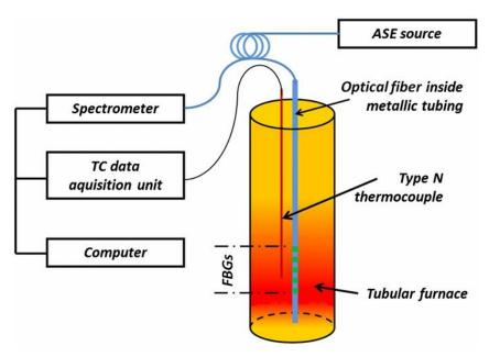
Figure 2. Annealing setup for FBG regeneration.
