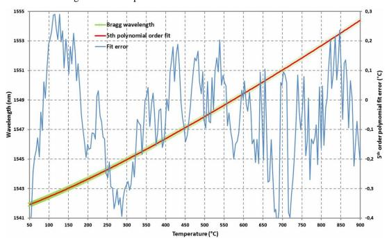
**Figure 6.** Fifth-order polynomial fit of the Bragg wavelength over a range of 850 °C.
