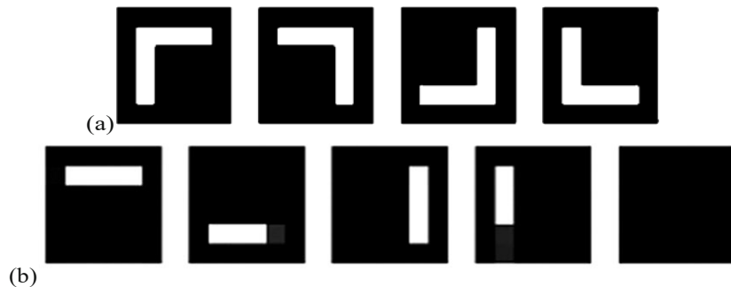
Fig. 15 Application of nonnegative tensor to image structure analysis: (a) initial binary images with corner elements; (b) recovered rank-1 nonnegative elements
