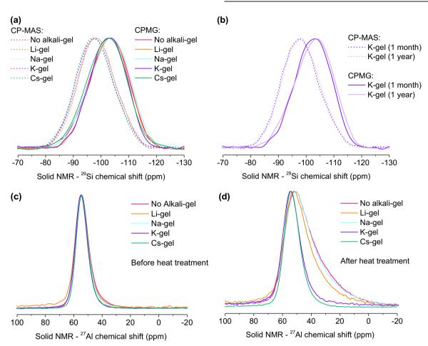
**Fig. 3** Solid-state NMR spectroscopy data. **a** <sup>29</sup>Si MAS CPMG and CP-MAS NMR spectra of each 3.5–5.5  $\mu$ m gel powders. **b** CP-MAS and CPMG NMR spectra of the 3.5–5.5  $\mu$ m gel powders altered 1 month and 1 year in a *K*-solution. **c**,**d** <sup>27</sup>Al MAS NMR spectra of each 3.5–5.5  $\mu$ m gel powders before heat treatment (**c**) and after heat treatment (300 °C) (**d**). All spectra are normalized to the same maximum height to facilitate their comparison
