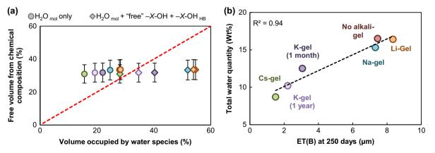
**Fig. 5** Data comparison. **a** Volume occupied by water species versus free volume from mobile species release (the error bars are smaller than the symbols for the volume occupied by water species). The red dashed line is the line x = y. **b** Total water quantity (from TGA) versus the B equivalent thicknesses at 250 days for each sample (the error bars are smaller than the symbols). The black dashed line is the linear regression between data. The error bars represent the standard deviation
