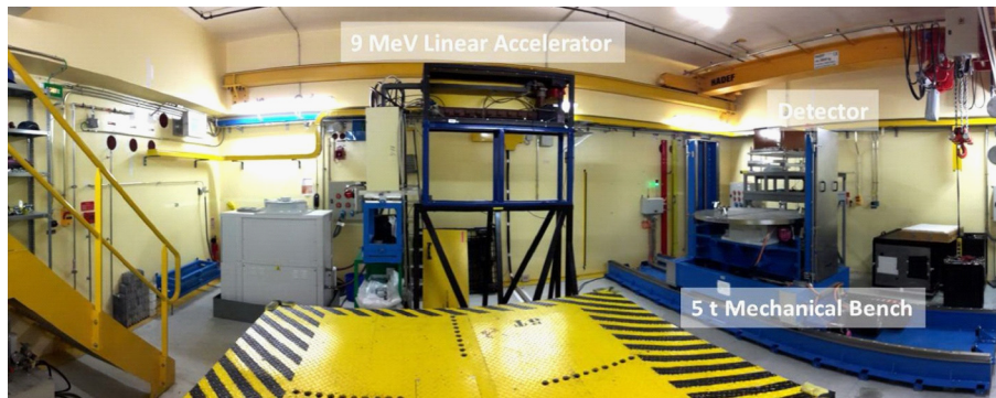
Fig. 13. The CINPHONIE cell hosting a high energy photon imaging system (the 9 MeV LINAC will be replaced soon by a 20 MeV LINAC), in the CHICADE basic nuclear facility, at CEA Cadarache.
