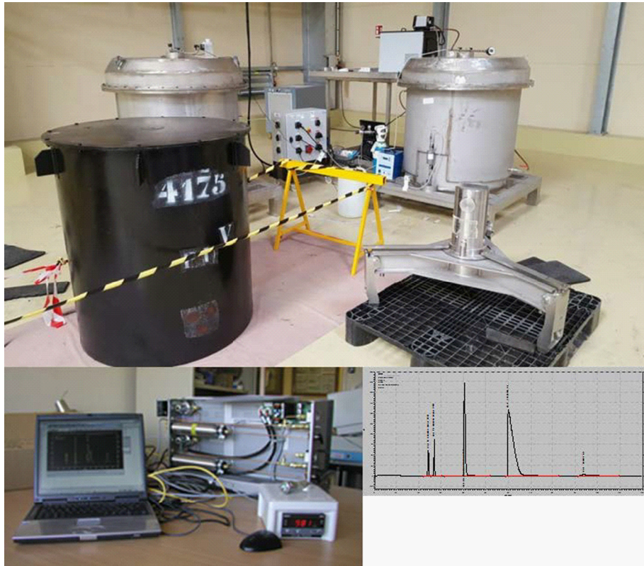
Fig. 11. Hydrogen degassing measurement station on 870 L packages (in black) at the CEDRA storage facility, CEA Cadarache. The containment enclosures (grey), adapted to the type of package, allow the accumulation of gases released from the package. A sample of the atmosphere of the chamber is then measured by gas chromatography (bottom left). The chromatogram (bottom right) shows the separation of the different gases in the atmosphere (hydrogen corresponds to the second peak).
