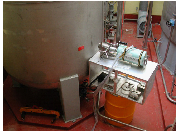
Fig. 5. Measurement of a vessel that contained contaminated effluents (HPGe detector).
