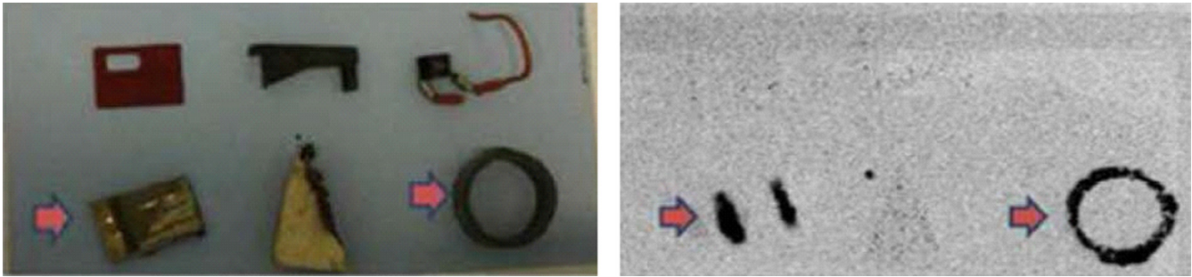
Fig. 9. Measurement of tritiated waste by digital autoradiography.
