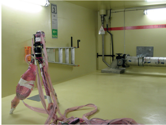
Figure 2 – La GAMPIX sur trépied durant les mesures en zone contrôlée. GAMPIX gamma camera on the tripod during measurements in the controlled area.
