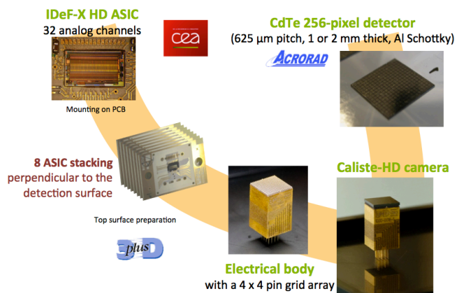
Fig. 1. Detailed components of a complete Caliste HD module.
