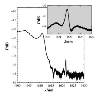
**Figure 3.** Fiber-to-fiber transmission (*T*) spectrum of a slotted PhC with a Q factor of 6500. Inset: zoom on the resonance.
