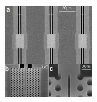
**Figure 2.** Scanning electron microscope (SEM) views of the fabricated slotted photonic crystal in polycrystalline diamond. **a)** SEM view of three photonic crystal cavities with their access waveguides maintained by nanotethers. **b)** Tilted view (45°) of a PhC and its access waveguide with the slot at the center. **c)** Tilted close view of a PhC with the 135-nm wide slot and its access waveguide.
