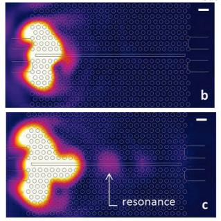
**Figure 4**. Optical images of the cavity at different wavelengths in false colors. For clarity, a schematic representation of the PhC is superimposed. **a)** waveguide transmission. **b)** cut off in the photonic band gap. **c)** cavity mode resonating at 1621.8 nm. Scale bar : 1μm.
