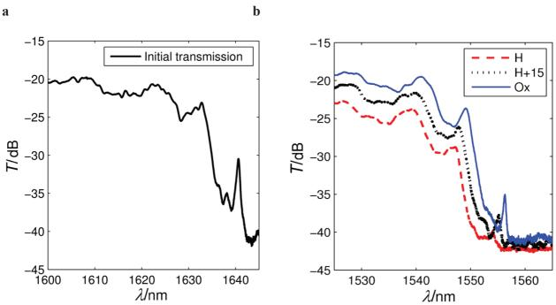
**Figure 6.** Transmission spectra of the photonic crystal cavities for different surface states. **a)** Spectrum at the end of the process. **b)** (dash red) hydrogenated PhC – (dot black) hydrogenated PhC after 15 days – (blue) oxidized PhC
