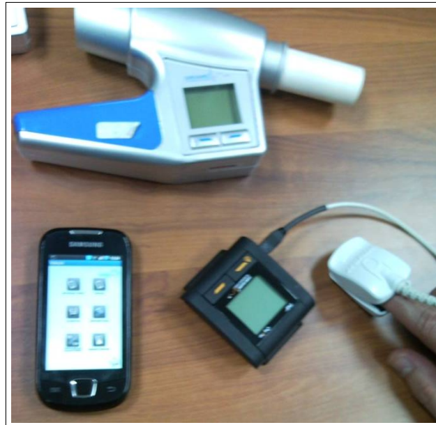
Figure 10. eHealth testbed snapshot. On the left, the Android cluster head of our setting running the Vida24 eHealth application that collects measurements from the oximeter device (on the right). Multiple devices can be paired and monitored, for example, the Spirometer device on the top of the figure.
