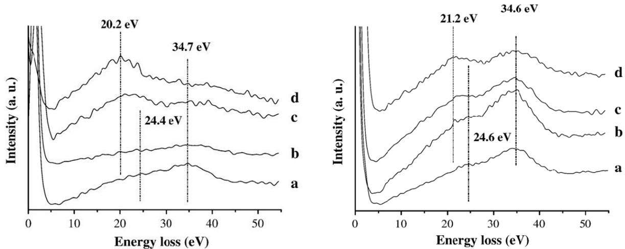
**Figure 12** XEELS spectra (left) after H<sub>2</sub> plasma; (right) after H<sub>2</sub> plasma and a short CVD growth (a) as introduced; (b) after a H<sub>2</sub> plasma at 720°C/15 min; (c) after a H<sub>2</sub> plasma at 940°C/15 min; (d) after a H<sub>2</sub> plasma at 940°C/45 min [95]
