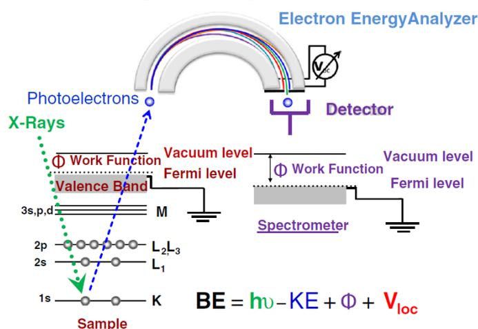
**Figure 1** XPS principle from [21].  $h\nu$  is the energy of incident photons, BE and KE are the binding and kinetic energies of photoelectrons,  $\phi$  the analyzer work function,  $V_{loc}$  the local electrical potential.
