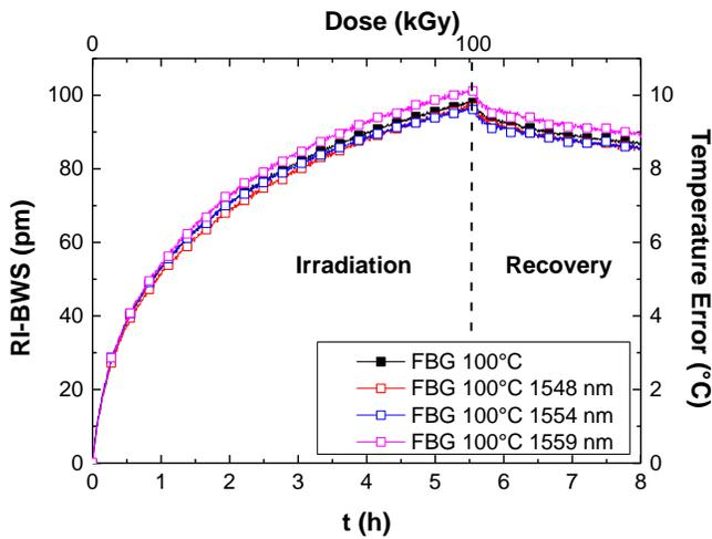
Figure 2: RI-BWS of a line of 3 FBGs ( $\lambda_B=1548$  nm; 1554 nm and 1559 nm) thermally treated at 100°C for 69 h after inscription during and after X-ray irradiation up to 100 kGy (5 Gy/s). On the right Y-axis the radiation induced error on the FBG temperature measurements is given.
