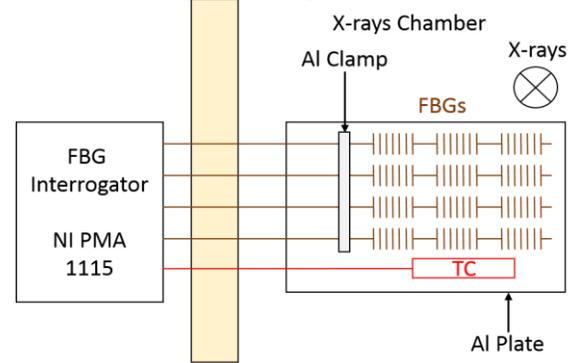
Figure 1. Experimental setup used for the X-ray irradiations: four fibers containing each three FBGs (identical inscription conditions – 3 different  $\lambda_B$ ) are fixed without stress on an Aluminium pad, with clamps and exposed to X-rays up to 100 kGy. Thermocouples (TC) measured the temperature evolution during irradiation.
