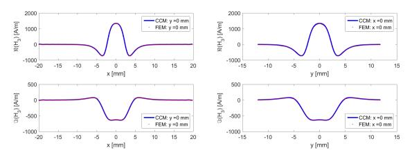
Figure 9: A sliceview of the comparison of the longitudinal component of  $H_w$  provided by CCM or by FE. On the top, cartographies of real parts are displayed, imaginary parts are placed at the bottom.
