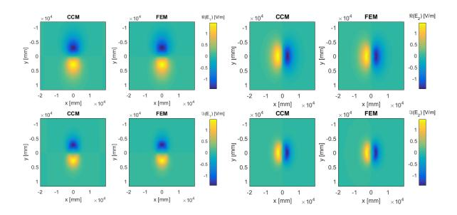
Figure 6: Comparison of the tangential components of **E** provided by the C method (CCM) or by Finite Element (FE). On the top, cartographies of real parts are displayed, imaginary parts are placed at the bottom.
