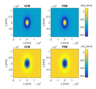
Figure 8: Comparison of the longitudinal component of  $H_w$  provided by CCM or by FE. On the top, cartographies of real parts are displayed, imaginary parts are placed at the bottom.
