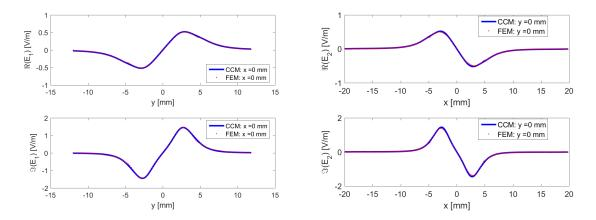
Figure 7: A sliceview of the comparison of the tangential components of **E** provided by CCM or by FE.
