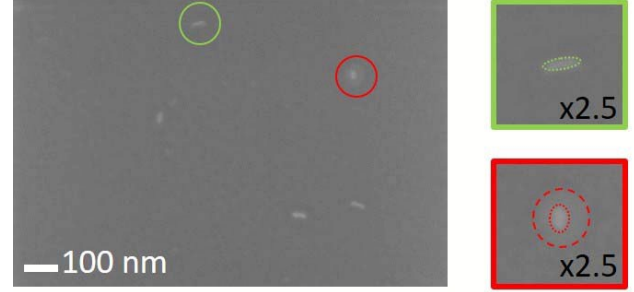
Fig. 6 SEM characterization of single GNRs in the absence (green circle) or after “over-illumination” (red circle). A pulse energy density of 2.5 \text{ mJ.cm}^{-2} was used with an incident polarization along the longitudinal axis of the GNR and at its longitudinal plasmon resonance wavelength. In the SEM images, dotted lines delineate the GNR from an additional halo observed following high power excitation. The dashed red line delineates a halo around the GNR. The GNR after illumination presents an aspect ratio of around 2. The GNR is clearly shorter than the one illuminated with a 125 \mu\text{J.cm}^{-2} pulse energy density as shown in Fig. 3.
