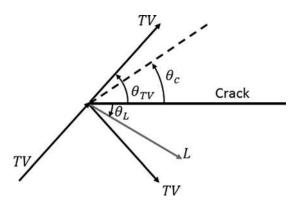
FIG. 8. Reflection of a transversal wave by a half-plane crack. An incident transversal wave gives rise to reflected transversal and longitudinal waves, which respect the Snell's law ( $\theta_L < \theta_{TV}$ ). For a transversal incidence below the longitudinal critical angle  $\theta_c$  ( $\theta_{TV} < \theta_c$ ), the longitudinal waves are no more reflected but laid on the crack surface.
