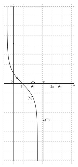
FIG. 2.  $\Gamma$  and the steepest descent path  $\gamma$  in the complex plane  $\lambda = \sigma + \tau$ .  $\theta_{\beta}$  is the real pole of the integral [Eq. (2)] and  $\bar{\theta}$  is its phase stationary point.
