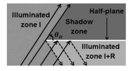
FIG. 3. Interaction of a plane wave with a semi-infinite crack embedded in an elastic homogeneous solid. Thick arrows, incident waves; dash arrows, reflected waves.
