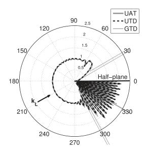
FIG. 9. Directivity pattern of the total field predicted by different models (GTD, UAT, and UTD) at  $r = 8\lambda_L$ ;  $\Omega_L = 90^\circ$ ,  $\theta_L = 30^\circ$ . Each circle represents an amplitude of the total field normalized by the incident amplitude.
