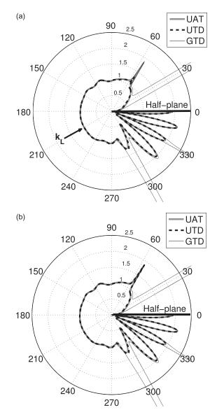
FIG. 5. Directivity pattern of the total field predicted by different models (GTD, UAT, and UTD) at  $r = 2\lambda_L$ ;  $\Omega_L = 90^\circ$ ,  $\theta_L = 30^\circ$ . (a) UTD model is the one found using Pauli–Clemmow method. (b) Modified UTD model. Each circle represents amplitude of the total field normalized by the incident amplitude.
