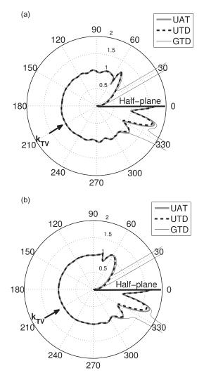
FIG. 6. Directivity pattern of the total field predicted by different models (GTD, UAT, and UTD) at  $r = 3\lambda_{TV}$  for  $\theta_{TV} = 30^{\circ}$ . (a)  $\Omega_{TV} = 90^{\circ}$ , (b)  $\Omega_{TV} = 60^{\circ}$ . Each circle represents amplitude of the total field normalized by the incident amplitude.
