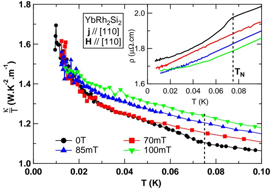
FIG. 5. (color online) Thermal conductivity of  $\text{YbRh}_2\text{Si}_2$  at low temperature below 0.1 T. In inset, the corresponding electrical resistivity. The dash line shows the Néel temperature at zero field.
