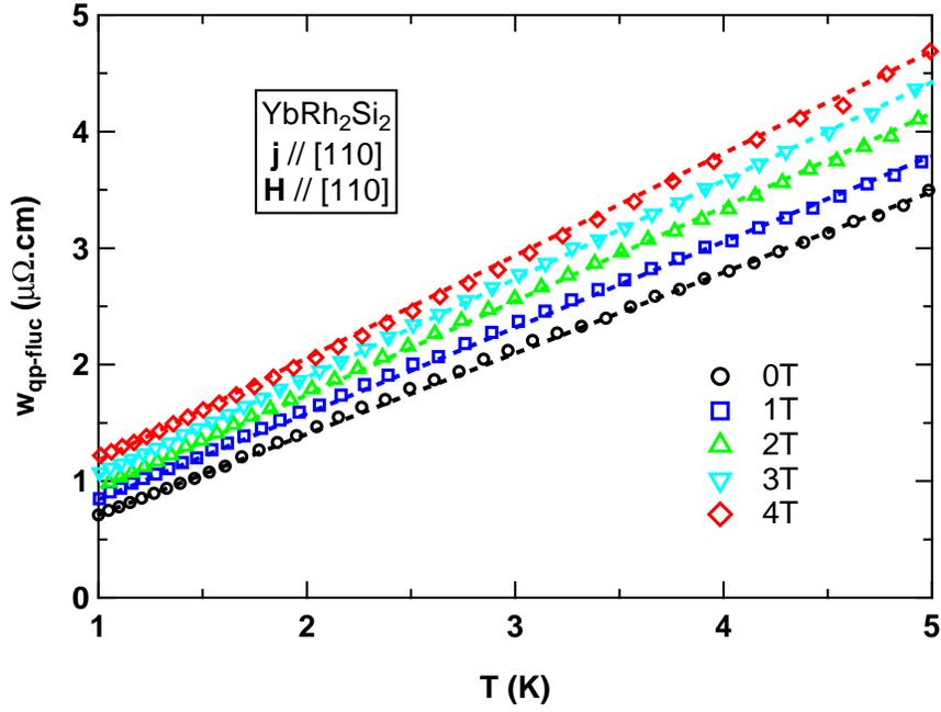
FIG. 7. (color online) Electronic thermal resistivity  $w_{qp-fluc}$  up to 5 K after subtraction of the electrical resistivity. For clarity, an offset has been added to each curve ( $+0.2 \mu\Omega.cm$  at each field step). Dashed lines are guides to the eyes.
