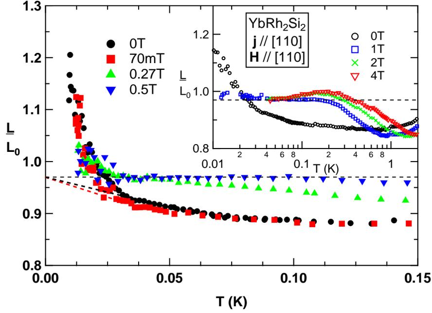
FIG. 2. (color online) Ratio  $L(T)/L_0$  at low temperatures below 1 T. The dashed lines are the extrapolation to  $L(0) = 0.97L_0$  when  $T > 30$  mK. In inset,  $L(T)/L_0$  at higher fields, which extrapolates also to 0.97 at low temperature.
