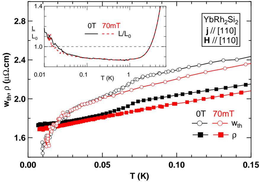
FIG. 1. (color online) Electrical resistivity (full squares) and thermal resistivity (open circles) of  $\text{YbRh}_2\text{Si}_2$  at 0 T (in black) and at 70 mT, close to  $H_c$  (in red) at low temperature. Clear anomalies are observed in zero field at  $T_N$ , and a new channel for heat transport appears below 30 mK (see text). *Inset*: Normalized ratio  $L(T)/L_0$  in the whole temperature range at 0 T and 70 mT.
