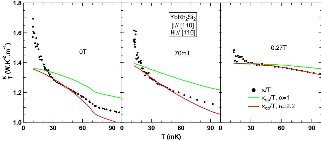
FIG. 3. (color online) Comparison of the electronic thermal conductivity using the expression 1 with  $\alpha = 1$  and  $\alpha = 2.2$ . The latter value was chosen to optimize the low temperature contribution of  $\kappa_{qp}$ .
