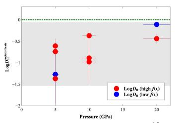
Fig. 3. Hydrogen partitioning between metal and silicate ( $logD_H^{net-sil}$ ) as a function of experimental pressure. Red and blue circles represent experiments performed at oxygen fugacities above IW-2 and below IW-3.5, respectively. The green dashed line at  $logD_H^{net-sil} = 0$  indicates the limit between lithophile (below) and siderophile behavior (above). The gray area encompasses the range of  $D_H$  values determined from our experiments, all of which indicate lithophile behavior.
