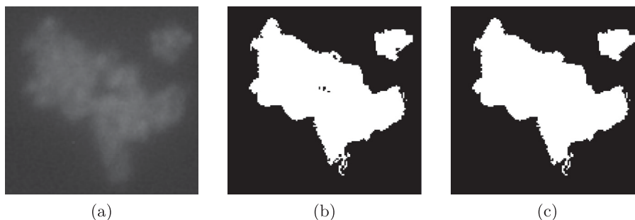
Fig. 6. Example of image thresholding and holes filling: original image (a), binarised image (b), and binarised image with holes filled (c).
