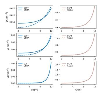
FIG. 1. Confined RNA density profile vs r the distance from the capsid center for various extrapolation lengths,  $\kappa^{-1}$ =10.0, 5.0, 2.0 nm for top to the bottom of the figure. The total monomer number is N=100(left), N=5000(right).
