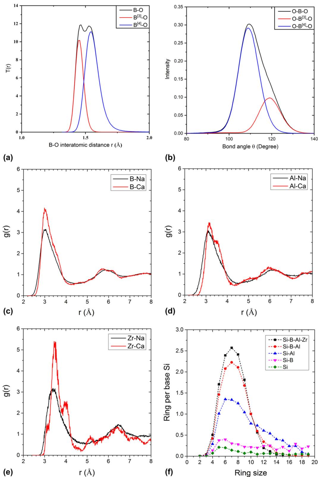
**Fig. 1** MD simulations of ISG structure. Deconvolution of **a** TCF of B-O and **b** BAD of O-B-O in the simulated ISG structure. **c** B-Ca/Na PDF. **d** Al-Ca/Na PDF. **e** Zr-Ca/Na PDF. **f** Ring size distribution calculated for different ISG glass formers
