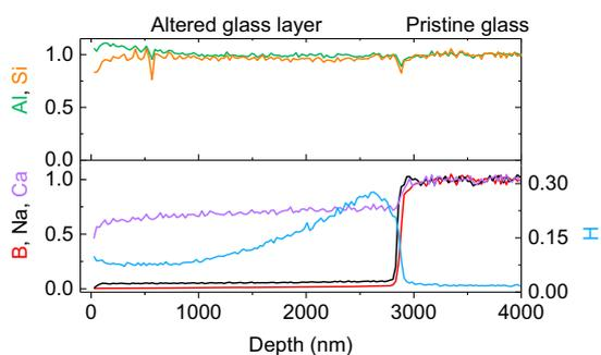
**Fig. 3** ToF-SIMS profiles. ToF-SIMS data obtained from ISG monolith altered for 25 days.  $Si, Al, B, Na,$  and  $Ca$  profiles are normalized to that of  $Zr$  to avoid matrix effects; the resulting data are normalized to that measured in pristine glass to provide quantitative information. The  $H$  profile is not normalized and is only used to locate the alteration front. The Methods section contains more information on data normalization
