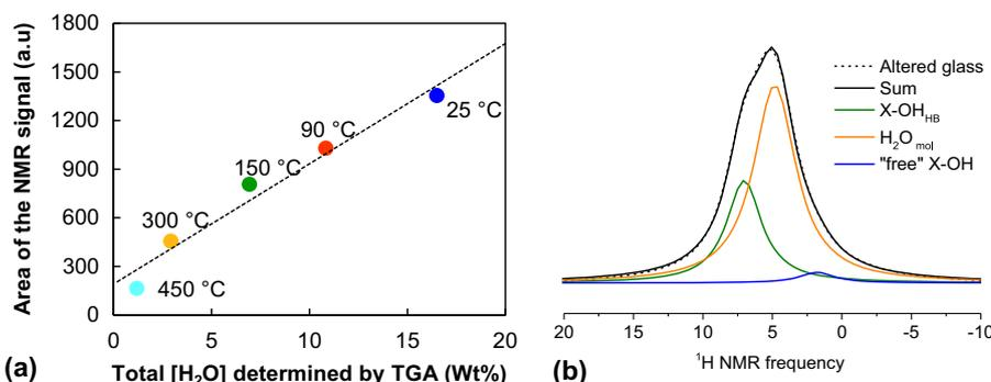
**Fig. 6** TGA and  $^1\text{H}$  NMR data comparison. **a**  $^1\text{H}$  NMR signal areas determined at various temperatures (25, 90, 150, 300, and 450 °C); these results are compared to the total water quantity ( $\text{H}_2\text{O}_{\text{mol}}$  + hydroxyl species) found by TGA at each temperature. They are well correlated. **b** Deconvoluted  $^1\text{H}$  NMR signal (at 25 °C)
