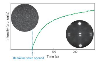
FIG. 5. Intensity of the k-space image recorded  $\sim 0.08 \text{ eV}$  below the Fermi level, as a function of the exposure time to the synchrotron beam. The k-space images recorded before and after exposure to beam are shown in the upper right and bottom left of the figure, respectively.
