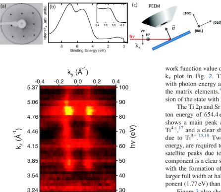
FIG. 2.  $k_y \cdot k_z$  map of the 2D state, located at  $k_x = 0 \ \text{\AA}^{-1}$ . The corresponding photon energy is also presented. Photon energy 30 to 100 eV with an inner potential of 14.5 eV (Ref. 15) and a WF of 4.5 eV gives  $k_z = 3.24$  to 5.37  $\ \text{\AA}^{-1}$ .
