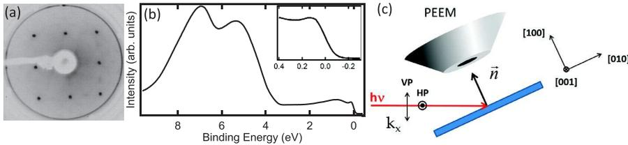
FIG. 1. (a)  $(1 \times 1)$  LEED (electron energy 66 eV). (b) Valence band spectrum taken at  $h\nu = 82.11$  eV showing gap states and metallic 2DEG at FL. (c) Geometry used for these  $k$ -PEEM experiments.
