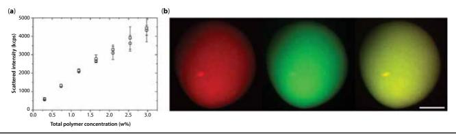
**Figure 5** (a) Homogeneity of chitosan-FITC:collagen-TRITC solutions assessed by light scattering measurements as a function of total polymer concentration in wt%. (b) Maximum intensity projection of a Z-stack of 41 successive slices of a hybrid microsphere imaged by confocal microscopy, with collagen labeled in red (left), chitosan in green (center) and overlay (right). The bar is 50 µm.
