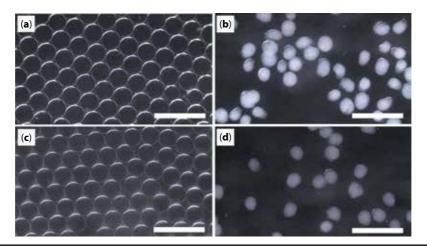
**Figure 2** Images of emulsion droplets and microspheres generated with the T-junction millifluidic device: (a) chitosan emulsion, (b) chitosan microspheres after ammonia vapors, (c) chitosan-collagen hybrid emulsion, (d) hybrid microspheres after ammonia vapors. Micrographs (a–d) were taken under darkfield illumination. Scale bar: 500 μm.
