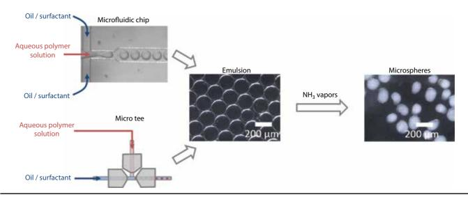
**Figure 1** General scheme for formation of microspheres: The initial emulsion is obtained with an acidic polymer solution and oil/surfactant mixture, with either a microfluidic chip or a MicroTee device. Microspheres are then obtained by solidifying the emulsion under ammonia vapors.
