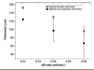
**Figure 4** Size of hybrid chitosan-collagen emulsion droplets (crossed open circle) and microspheres after ammonia vapors (solid circles) as a function of oil flow rate at constant chitosan solution flow rate (0.002 ml.min $^{-1}$ ). Chip 100  $\times$  100  $\mu m^2$  cross design.
