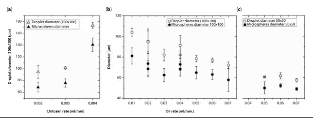
Figure 3 Size of emulsion droplets (open symbols) and microspheres after ammonia vapors (solid symbols): (a) as a function of chitosan solution flow rate at constant oil flow rate (0.02 ml.min<sup>-1</sup>) and (b) as a function of oil flow rate at constant chitosan solution flow rate (0.002 ml.min<sup>-1</sup>). The emulsion was obtained on a microfluidic chip with a  $100 \times 100 \, \mu m^2$  (a, b) or  $50 \times 50 \, \mu m^2$  (c) cross design.
