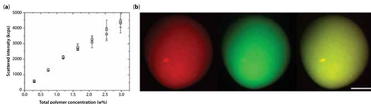
**Figure 5** (a) Homogeneity of chitosan-FITC:collagen-TRITC solutions assessed by light scattering measurements as a function of total polymer concentration in wt%. (b) Maximum intensity projection of a Z-stack of 41 successive slices of a hybrid microsphere imaged by confocal microscopy, with collagen labeled in red (left), chitosan in green (center) and overlay (right). The bar is 50  $\mu\text{m}$ .
