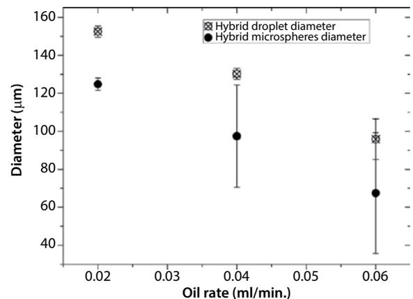
**Figure 4** Size of hybrid chitosan-collagen emulsion droplets (crossed open circle) and microspheres after ammonia vapors (solid circles) as a function of oil flow rate at constant chitosan solution flow rate ( $0.002 \text{ ml}\cdot\text{min}^{-1}$ ). Chip  $100 \times 100 \mu\text{m}^2$  cross design.
