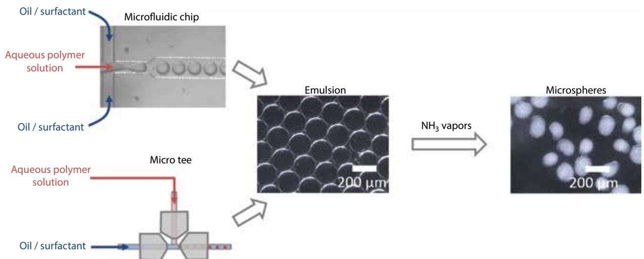
**Figure 1** General scheme for formation of microspheres: The initial emulsion is obtained with an acidic polymer solution and oil/surfactant mixture, with either a microfluidic chip or a MicroTee device. Microspheres are then obtained by solidifying the emulsion under ammonia vapors.
