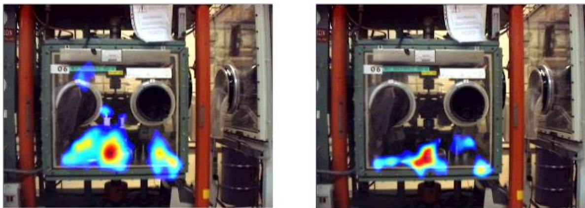
Figure 1 : Image of a glove box containing a press – on the left, image from a gamma camera equipped with a pinhole; on the right, image from a gamma camera equipped with a coded mask.
