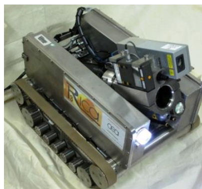
Figure 5: Example of a module grouping instruments for the location and radiological characterization of hot spots (DUCROS, HAUSER, Majhoubi, & GIRONES, 2016)
