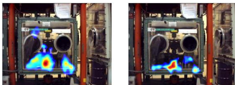
Figure 4: Example of gamma images (Aladin imager equipped with a CSi detector) – on the left, pinhole optics, on the right coded optical mask. The situation shown is 241 Am contamination in a glove box containing a nuclear fuel pellet press.
