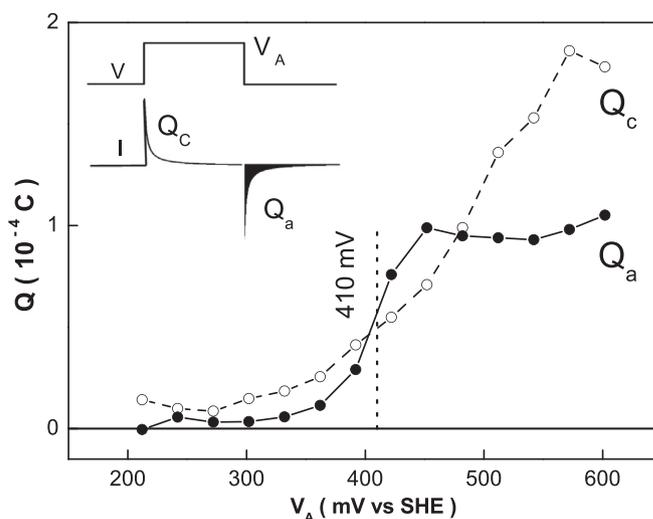
Fig. 5. Cathodic charge (full symbols), and anodic charge (empty symbols), as a function of the anodic charging potential, for a cleaved (001)  $\text{Sr}_2\text{IrO}_4$  single crystal ( $7.6 \cdot 10^{-3} \text{ cm}^2 \times 50 \mu\text{m}$ ) in 1 M KOH.
