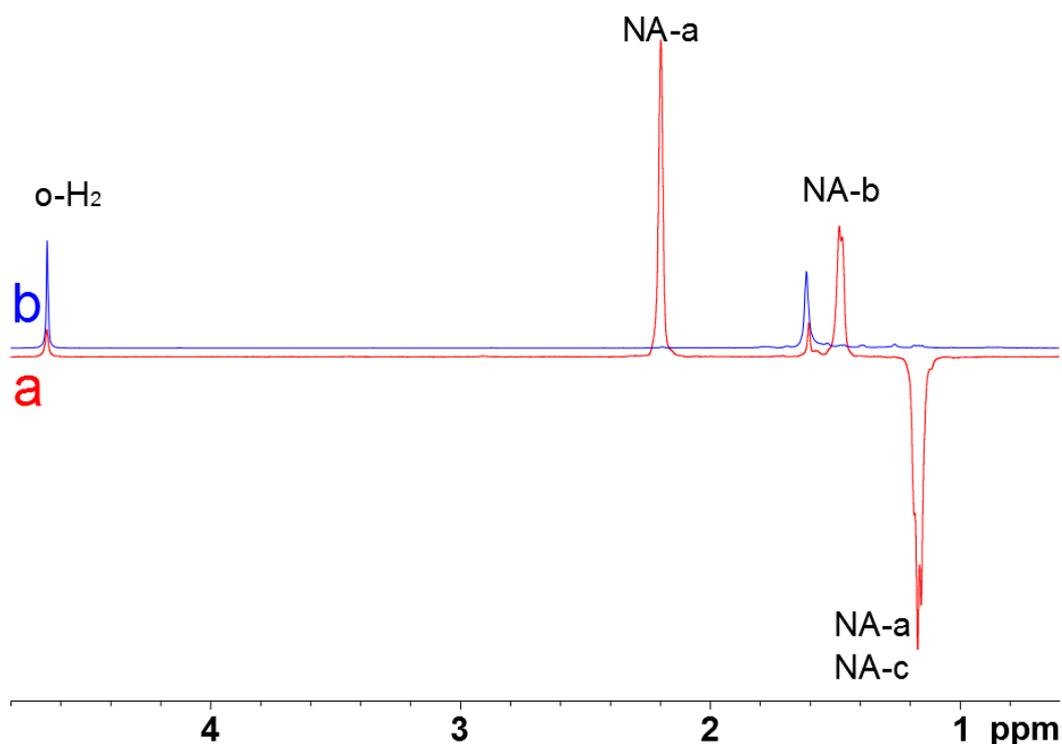
**Figure 3.** Upfield region of the one-scan  $^1\text{H}$  NMR spectrum of **1** (0.3 mM), (a) after introduction of para-hydrogen and (b) 6 minutes later. A  $45^\circ$  readout pulse has been used.
