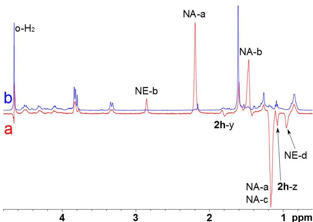
**Figure 2.** Upfield region of the one-scan <sup>1</sup>H NMR spectrum of **2h** (1 mM) in the presence of **1** (0.3 mM), (a) after the introduction of para-hydrogen and (b) 6 minutes later. A 45° readout pulse has been used.
