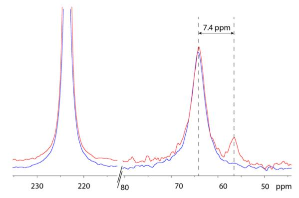
**Figure 5.** <sup>129</sup>Xe NMR spectra before, in blue, and after, in red, partial hydrogenation of **4**. A line broadening of 80 Hz has been applied prior to Fourier transformation.
