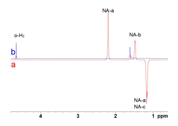
**Figure 3.** Upfield region of the one-scan <sup>1</sup>H NMR spectrum of **1** (0.3 mM), (a) after introduction of para-hydrogen and (b) 6 minutes later. A 45° readout pulse has been used.
