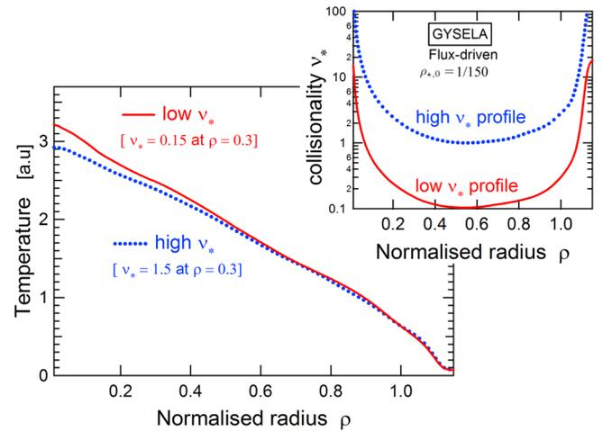
**Figure 9.** Temperature and collisionality profiles of figure 8 in banana and plateau regimes for the otherwise same plasma parameters. Confinement degrades and the central temperature drops by about 10% as the staircase pattern starts disappearing at higher collisionality.
