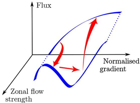
**Figure 14.** Example of breakdown of local flux-gradient relation: as the system evolves (red arrows) the flux-gradient landscape is modified by a third control parameter (here zonal flow strength) from single-valued to multi-valued and back to single-valued at large normalised gradient drive.
