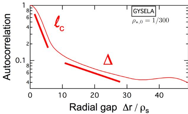
**Figure 3.** Autocorrelation of the electrostatic potential. Two slopes are found: the local autocorrelation length  $\ell_c \sim 6 \rho_s$  is microscale, the mesoscale is indicative of avalanches and therefore noted  $\Delta$  (see section 2.4.1).
