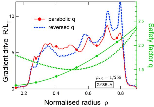
**Figure 21.** Same data as in figure 5, averaged between 4000 and 4610  $a/c_s$ . Two situations are compared: all other parameters being equal, the safety factor profile is either parabolic or reversed. A weak response of the central staircase step to the reversed magnetic shear is observed.
