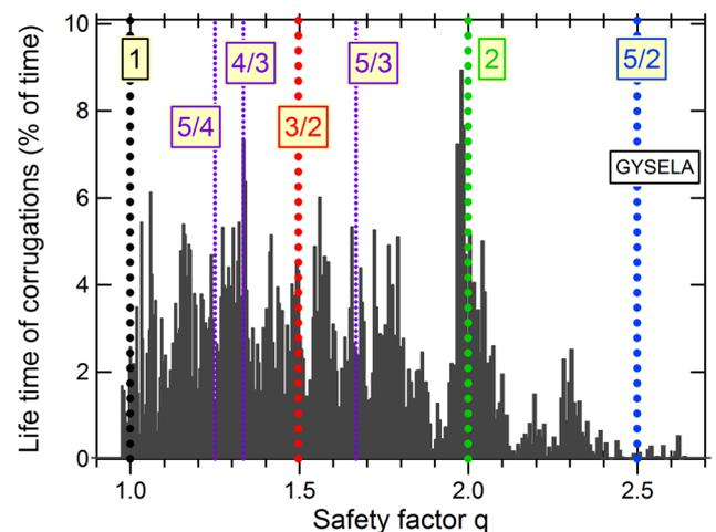
**Figure 20.** Statistics from figure 18 of the time staircase microbarriers (tracked as temperature corrugations) have spent in the vicinity of given  $q$  values, between  $t = 500$  and  $3900 a/c_s$ .
