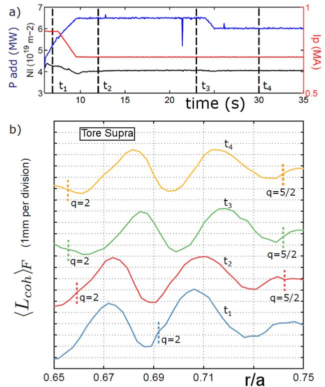
**Figure 23.** Experimental coherence length profiles  $\langle L_{\text{coh}} \rangle_F$  of density fluctuations at times  $t_1$  through  $t_4$ .
