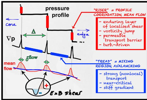
Figure 1. The  $\mathbf{E} \times \mathbf{B}$  staircase, schematic view.
