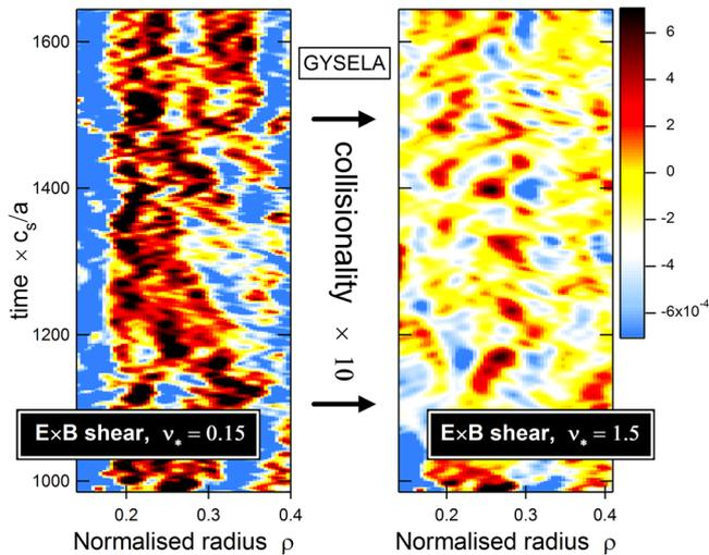
**Figure 8.** Impact of collisional dissipation on the  $\mathbf{E} \times \mathbf{B}$  staircase. The pattern exists in the low-collisional banana ( $\nu_* = 0.15$ ) limit of magnetised plasma turbulence and starts disappearing at the plateau transition ( $\nu_* = 1.5$ ).
