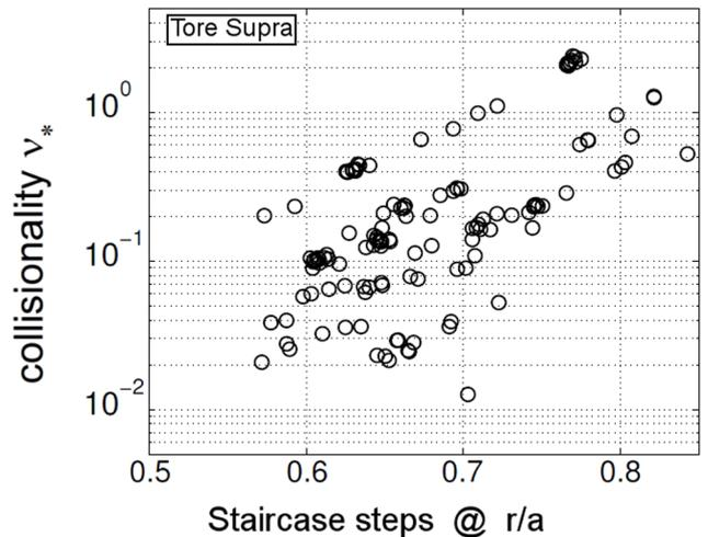
**Figure 7.** Experimental observation of staircase corrugations as a function of collisionality and radial location in Tore Supra. Staircases have only been observed so far in the low-collisional banana regime, supporting calculation predictions (see figure 8).
