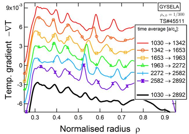
**Figure 22.** How the meandering of the  $\mathbf{E} \times \mathbf{B}$  staircase leads to its seeming disappearance when time integration is large. Radial coarse-graining leads to the same result. This sets constraints on experimental time and space resolution in order to resolve the staircase structure. For clarity, the curves at different times have been vertically offset from each other.
