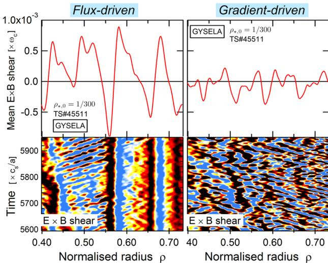
**Figure 11.** The mean  $\mathbf{E} \times \mathbf{B}$  shear, averaged over  $0.3$  ms ( $1$  collision time at  $\rho = 0.5$ ) is shown in both flux- and gradient-driven computations that display comparable turbulence intensities (see figure 26). No perennial structures genuinely endure in the gradient-driven approach, mean components are vanishing and the staircase pattern is lost.
