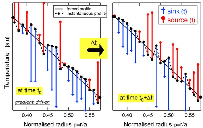
Figure A2. Evolution, as the temperature fluctuates, of the adaptive gradient-driven source/sink equation (A.2) from one time step  $t_0$  to a next  $t_0 + \Delta t$ . The gradient-driven forced profile (solid line) is computed from the flux-driven mean  $T_{F-D}$  profile in figure 24 and coincides with the flux-driven ‘ambient mean profile’, as defined on page 3. For clarity, only a zoom between  $\rho = 0.37$  and  $0.57$  is shown.
