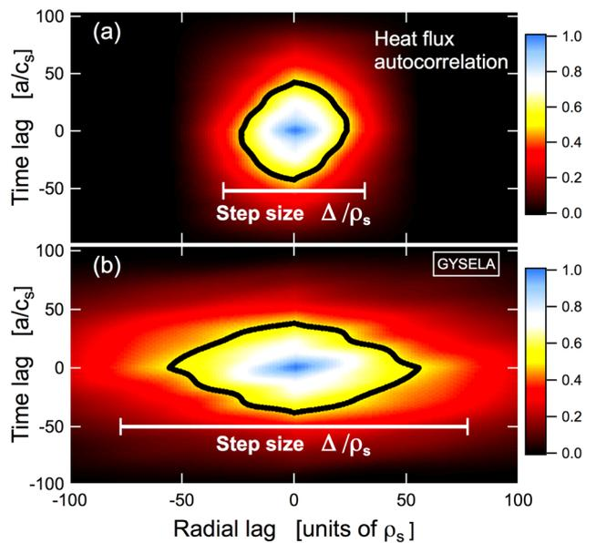
**Figure 16.** Autocorrelation of the turbulent heat flux in two separate radial regions of the plasma, at the same time, during 100  $a/c_s$ : case (a) in-between two staircase steps distant of  $\Delta = 58 \rho_s$  and case (b) distant of  $\Delta = 153 \rho_s$  (shown as white interval). In both cases the full width at half maximum (black contour), a measure of the radial coherence of heat transport, tracks well the local staircase step width.
