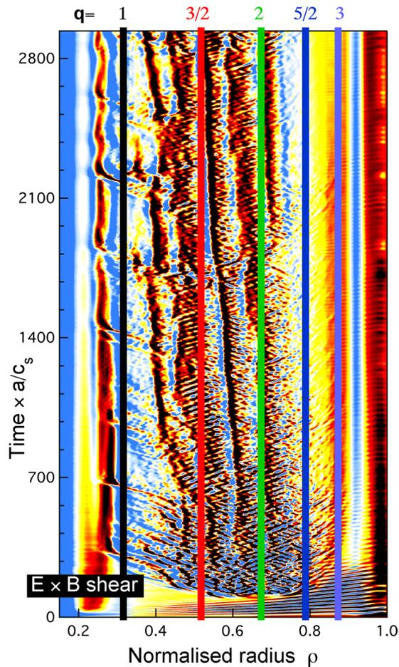
**Figure 18.** Same data as in figure 2 where the fixed locations of low-order  $q = 1, 3/2, 2, 5/2$  and  $3$  rationals are superimposed on top of the  $\mathbf{E} \times \mathbf{B}$  shear, marking the staircase steps. No clear connection between low-order  $q$  rationals and staircase microbarriers can be inferred.
