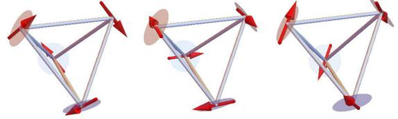
FIG. 1. (Color online) Sketch of the three configurations corresponding to the Palmer-Chalker ground state. The local XY planes perpendicular to the  $\langle 111 \rangle$  axes are indicated by colored disks. In the Palmer-Chalker configurations, spins are pairwise anti-parallel, and collinear with an edge of the tetrahedron. These configurations can be described as chiral spin crosses.
