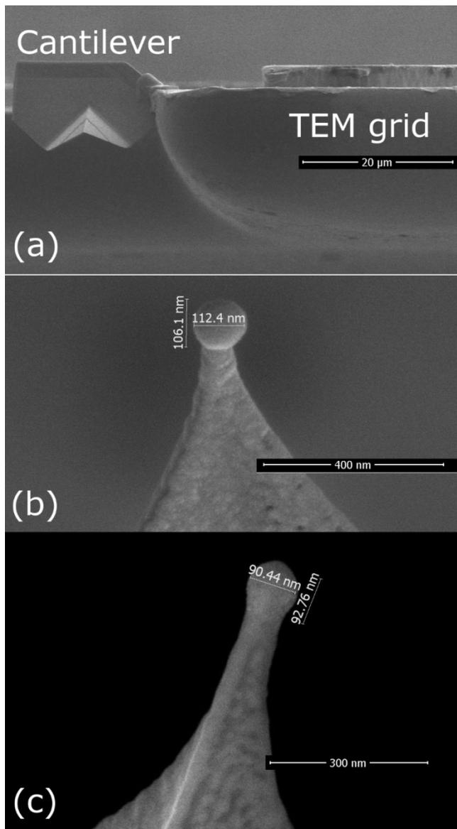
**Figure 3:** SEM micrographs of the cobalt nanospheres grown on cantilever tips for STEM-EELS and Electron Holography experiments. (a) Cantilever pyramid tip welded to a TEM grid. (b, c) Cobalt nanospheres grown by FEBID on the apex of the cantilever already attached to the TEM grid. The diameter of the nanospheres shown is 110 nm (b) and 90 nm (c).
