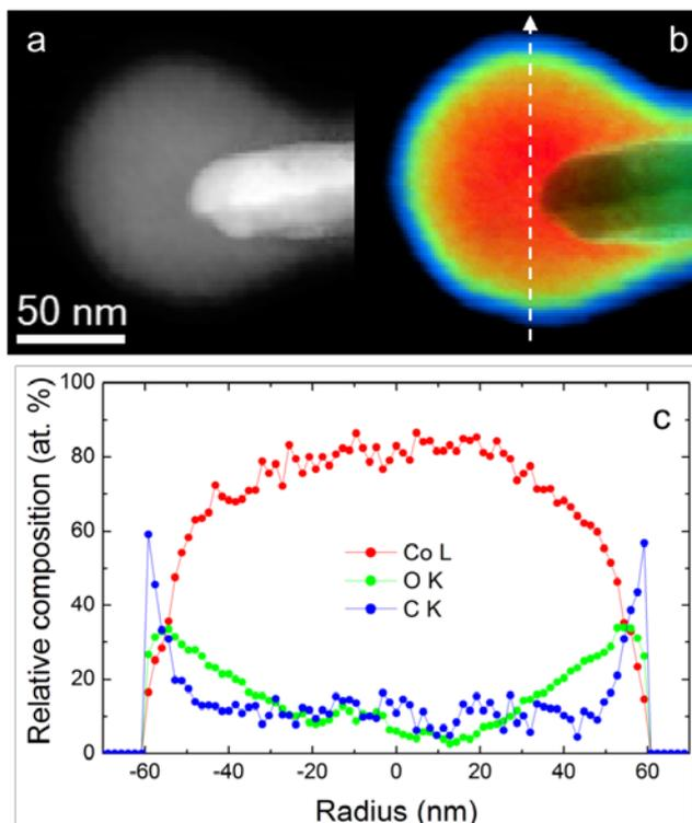
**Figure 4:** STEM-EELS compositional analysis of the cobalt nanosphere with 110 nm of diameter. (a) Reference image in Z contrast. (b) Colored chemical map, including the relative compositions of Co (red), O (green) and C (blue). (c) Compositional line profile extracted along the white arrow in (b).
