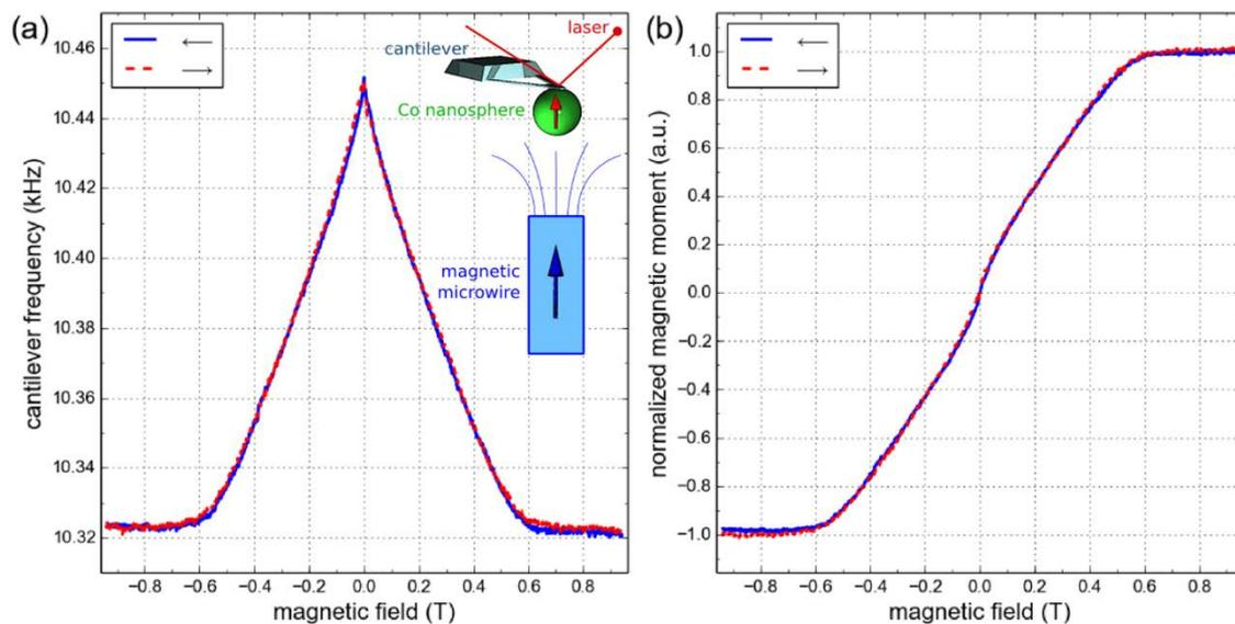
**Figure 6:** Cantilever magnetometry of a 500 nm diameter cobalt nanosphere. (a) Raw data of the cantilever frequency vs. applied magnetic field. Inset: Sketch of the cantilever magnetometry set-up. (b) Extracted magnetization curve.
