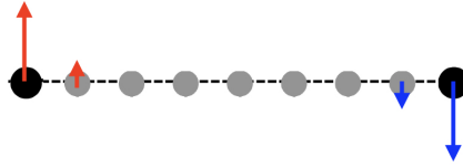
Figure 4: (Color online) One-dimensional wire: Majorana states form with MP vectors pointing in opposite direction at the two ends.
