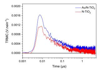
Figure 4. TRMC signal of  ${\rm N\text{-}TiO}_2$  and  ${\rm Au/N\text{-}TiO}_2$  obtained by irradiation at 450 nm.
