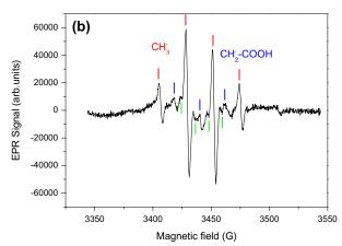
**Figure 7.** EPR spectra of (a) Au/TiO<sub>2</sub> and (b) N-TiO<sub>2</sub> in presence of acetic acid recorded at 77 K, and irradiated at  $\lambda = 365$  nm.
