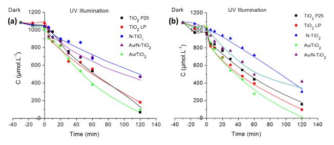
**Figure 5.** Photocatalytic decomposition of acetic acid (a) and propionic acid (b) under UV illumination for pure and modified TiO<sub>2</sub> samples (the lines are only guides for the eyes).
