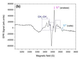
**Figure 8.** EPR spectra of (a)  $Au/TiO_2$  and (b) N-TiO<sub>2</sub> in presence of propionic acid recorded at 77 K, and irradiated at  $\lambda = 365$  nm.
