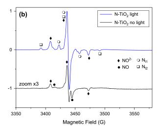
**Figure 2.** EPR spectra observed for dry photocatalysts powder without (dark curves) and with (blue curves) *in situ* UV-visible (halogen-lamp) irradiation at T = 60 K. (see exp. section for details). (a) Au modified sample, (b) N-doped sample.
