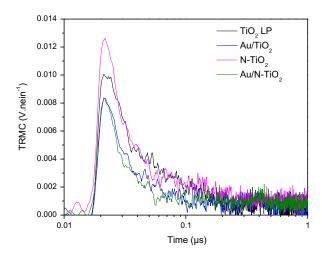
**Figure 3.** TRMC signal of pure and modified  ${\rm TiO_2}$  obtained by irradiation at 355 nm.
