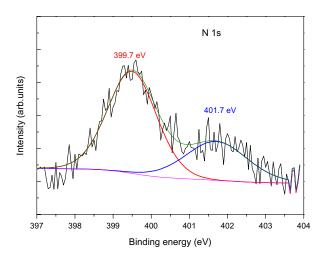
Figure 1. XPS spectrum of N-TiO<sub>2</sub> powder.
