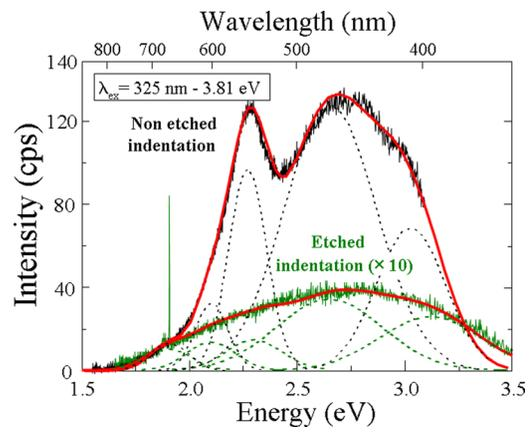
FIG. 2. (Color online) Comparison of photoluminescence under  $3.81 \text{ eV}$  excitation for non etched ( $10 \mu\text{W}$  laser power) and etched indentation ( $1 \text{ mW}$  laser power). The spectrum of etched indentation is enlarged by a factor 10 in order to show its Gaussian components. Signal of etched indentation is e.g., about 30 times stronger than the one of etched surface shown on Figure 1.
