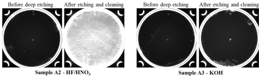
Fig. 5. DMS observations before and after deep etching of the whole surface of 50 mm diameter samples (Samples A2 and A3). Identical lighting and detection conditions. Bright spots in the center and on the top are fiducials.
