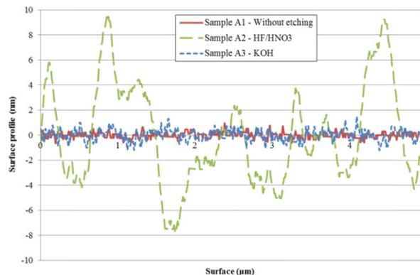
Fig. 7. Surface profiles obtained from the AFM measurements on the surfaces etched with HF/HNO<sub>3</sub> solution or KOH solution and on the polished surface without etching
