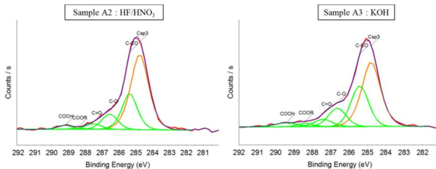
Fig. 8. Carbon high resolution XPS spectra obtained after cleaning on a sample etched with a HF/HNO<sub>3</sub> solution (Sample A2) and on a sample etched with a KOH solution (Sample A3)
