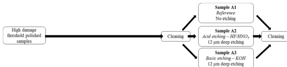
Fig. 1. Preparation of the samples for surface characterizations
