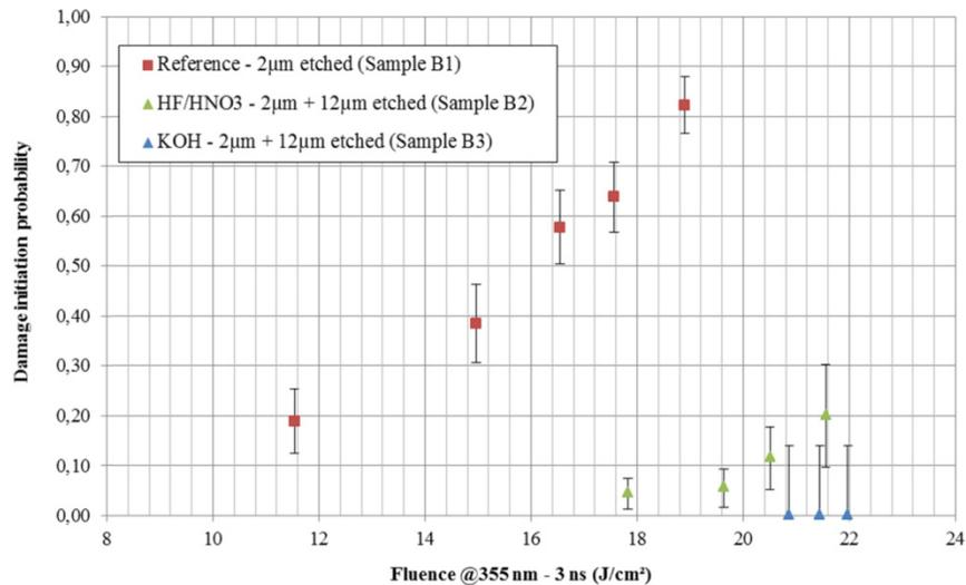
Fig. 11. Laser damage probability versus laser fluence at 355 nm and 3 ns for the scratched and etched samples (B1: red squares – reference, B2: green triangles – HF/HNO<sub>3</sub> etching, B3: blue diamonds – KOH etching).
