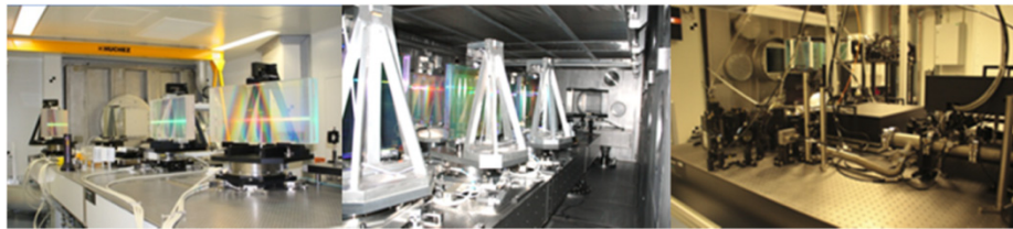
Fig. 9. 1st stage of compression in air (left), 2nd stage of compression in the vacuum vessel (center) and compression diagnostics table (right).
