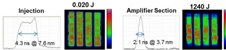
Fig. 6. Sub-apertures beam amplification up to 1.24 kJ.
