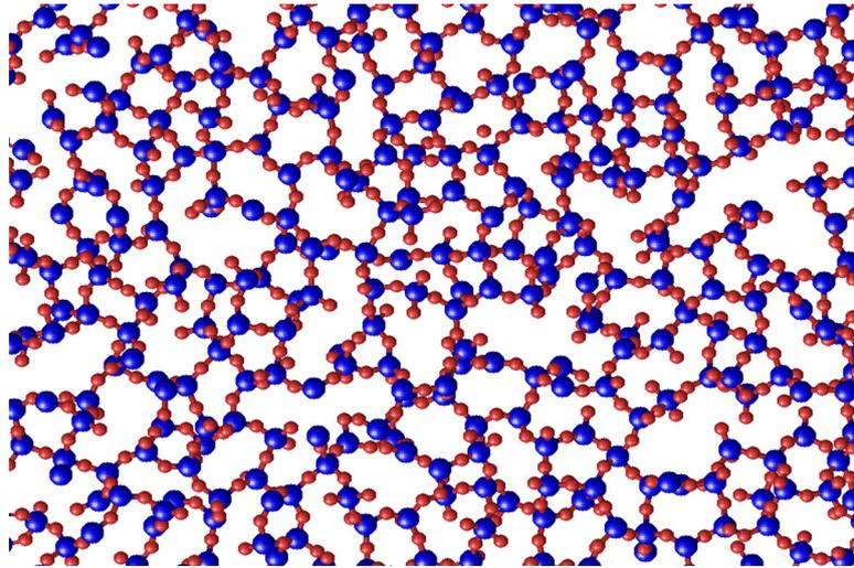
**Figure 7.** A sectional view of a 3D molecular dynamics simulation which shows a typical amorphous silica ( $\text{SiO}_2$ ) system. Blue spheres represent Si atoms, and red spheres represent O atoms.
