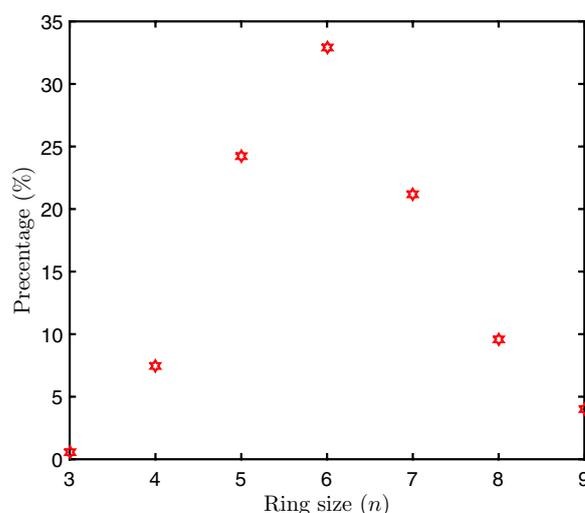
**Figure 10.** Distribution of rings as per molecular dynamics simulations of pure-amorphous silica [43, 78–81] with  $\sim 5000$  atoms. Simulations invoke the Vashishta *et al* potential [82, 83]. The independent variable,  $n$ , concerns the ring size. An  $n$ -member ring has  $n$  Si atoms and one O atom between each of the Si atoms (for a total of  $n$  Oxygen atoms in the ring).
