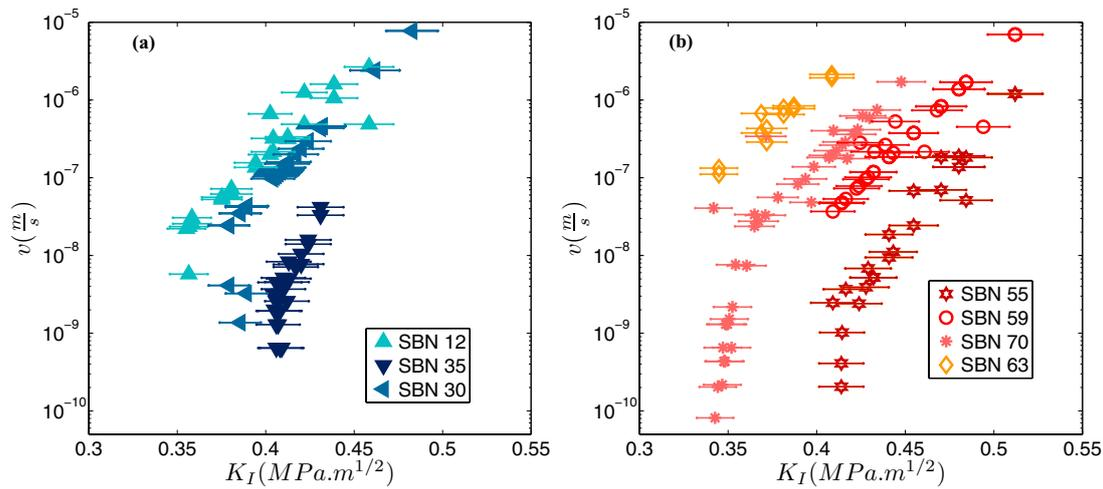
**Figure 20.** Velocity,  $v$ , as a function of stress intensity factor,  $K_I$ , for 7 different SBN glasses with two different  $K_{SBN}$  values: (a) 2.5 and (b) 4.5. Reprinted from [65], with permission from Elsevier. Table 12 provides the chemical composition of the glasses.
