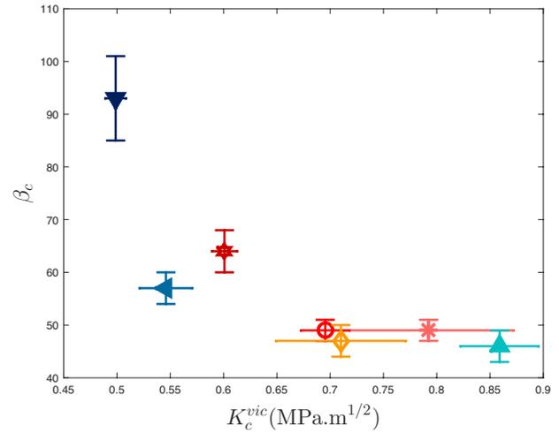
**Figure 28.** Slope in Region I ( $\beta_c$ ) as a function of the Vickers fracture toughness,  $K_c^{vic}$ , using equation (36).
