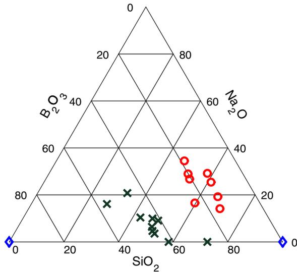
**Figure 14.** Ternary diagram of the location of the points defined in tables 6 and 8. Blue diamonds are for the extremities; pure silica and pure boron oxide [60, 122]. Red circles indicate data from [60]. Green × indicate data points from [122].
