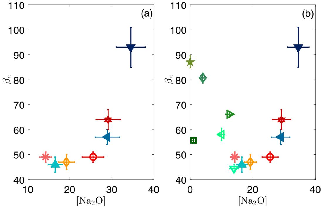
**Figure 24.** The slope in Region I ( $\beta_c$ ) as a function of [Na<sub>2</sub>O]. Panel (a) displays the SBN samples of Barlet *et al* [65]. Panel (b) displays all samples presented in table 12. It should be noted that Wiederhorn *et al* [1] glasses include multiple glass modifiers and glass intermediates and are more complex than the SBN samples of Barlet *et al* [65]. Reprinted from [65], with permission from Elsevier.
