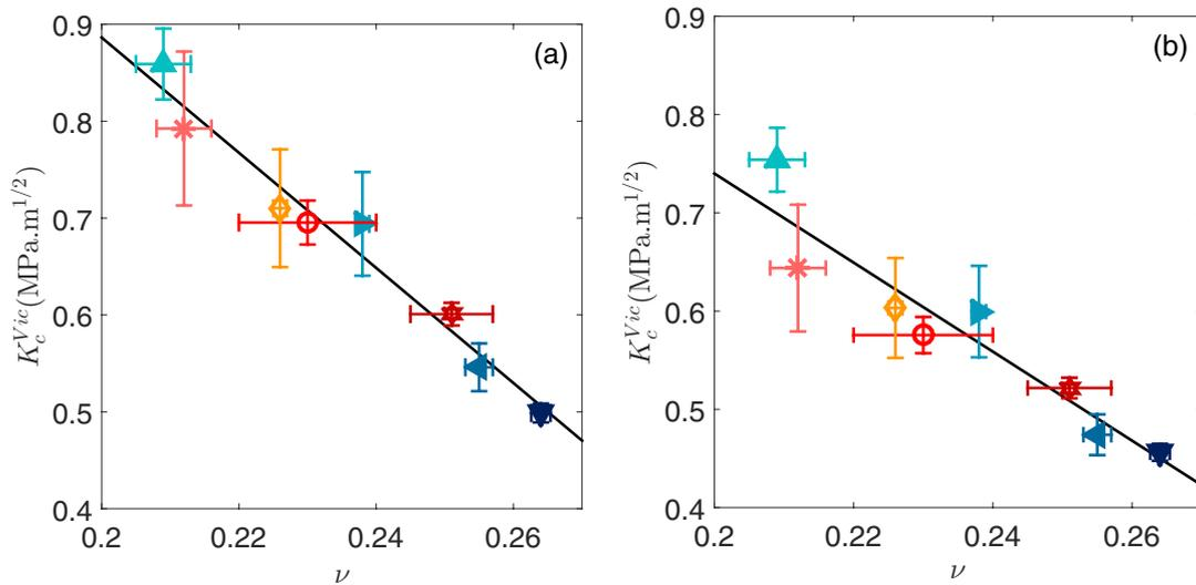
**Figure 18.** Vickers fracture toughness,  $K_c^{Vic}$ , as a function of Poisson’s ratio,  $\nu$  using (a) equation (36) and (b) equation (37). Symbols represent different types of SBN glasses (see table 11 for the key). Each point arises from an average over maximum loads of 50 and 100 g which have well formed cracks.
