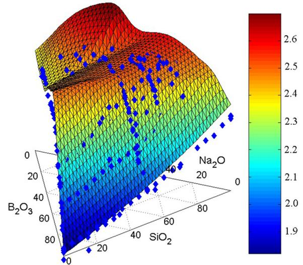
**Figure 13.** Density of SBN glasses as a function of their mole % of  $SiO_2$ ,  $B_2O_3$ , and  $Na_2O$ . The surface is from Inoue *et al* [97] first order mixing equations and parameters. The color bar indicates the density of the SBN glass in g/cc. Blue diamonds indicate experimental data. Reprinted from [60], with permission from Elsevier.
