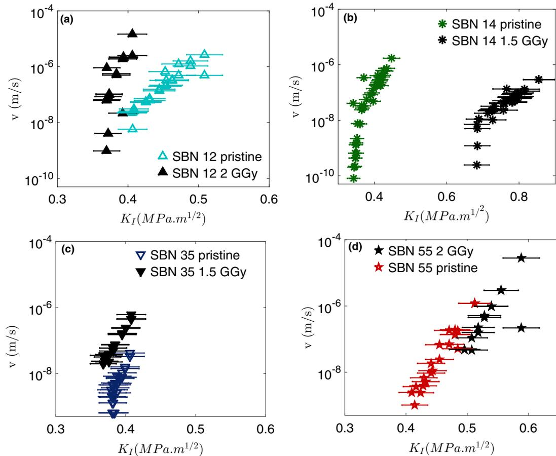
**Figure 29.** Evolution of the stress corrosion cracking curves before and after electron irradiation. Images plot the velocity,  $v$ , as a function of the stress intensity factor,  $K_I$ , for (a) SBN12, (b) SBN14, (c) SBN35 and (d) SBN55.
