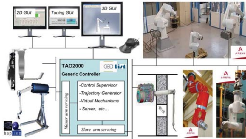
Figure 2. TAO2000 controller software architecture.
