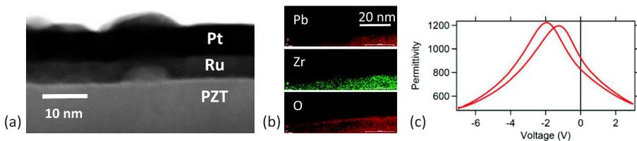
FIG. 1. (a) High-resolution bright field TEM cross-section of the as-grown Pt/Ru/PZT interface. (b) Pb, Zr, and O cross-sections of the Ru/PZT interface and (c) permittivity-voltage characteristic.
