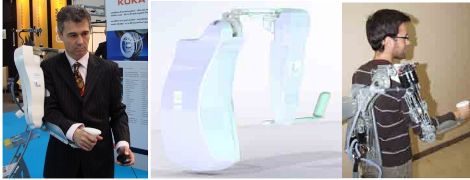
Fig 1. ABLE 4D exoskeleton actuated by screw-and-cable actuators (SCS actuator)
