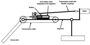
Fig 7. Embedded SCS principle
