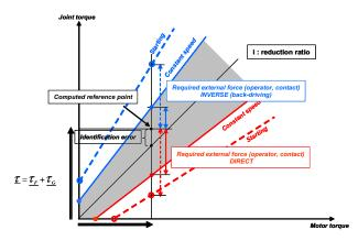
Fig 13. Actuator input-ouput force transmission diagram (in a quasi-static state)
