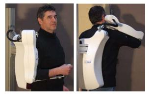
Fig 1. CEA-LIST 4 axis exoskeleton actuated by screw-and-cable actuators (SCS actuator)
