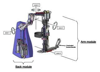
Fig 12. ABLE - 4 axis architecture
