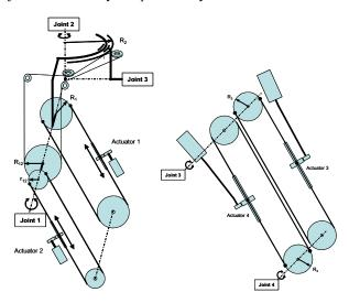
Fig 11. ABLE - 4 axis actuator kinematics: left, back module (Joints 1&2); right, arm module (Joints 3&4)
