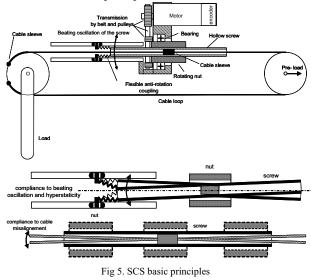
On the schemes (Fig 5) we can first see a general view of the actuator. A rotative joint is driven by a standard pushpull cable. On one side, the cable is driven by a ball-screw which translates directly in its nut (the screw is locked in rotation thanks to rollers moving into slots). The nut is rotating in a fixed bearing and is driven by the motor thanks to a belt transmission. Alternatively, a direct-drive pan-cake motor has been used in other applications as it is shown on Fig 6.
