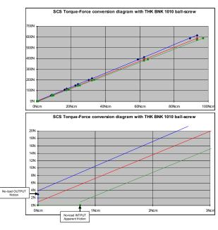
Fig 14. A typical SCS force transmission diagram
