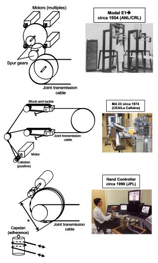
Fig 2. Landmarks in torque amplification for back-drivable electrical master-slave telemanipulator (EMSM)
