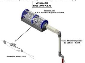
Fig 3. Virtuose 6D the first six axis force feedback master arm powered by screws and cables
