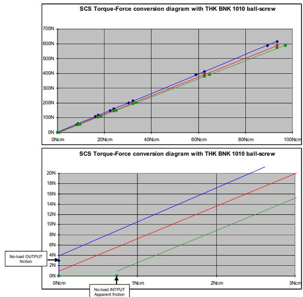
Fig 14. A typical SCS force transmission diagram
