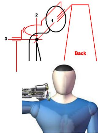
Fig 10. ABLE - 4 axis shoulder kinematics
