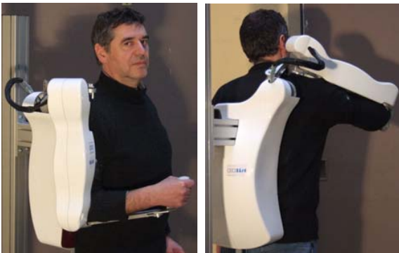
Fig 1. CEA-LIST 4 axis exoskeleton actuated by screw-and-cable actuators (SCS actuator)
