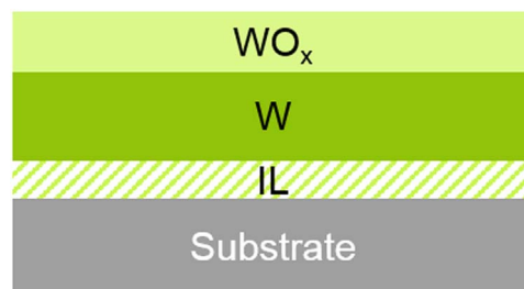
Fig. 8. Schematic representation of a F-free W film based on physicochemical characterizations realized in this study.
