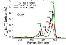
**Figure 3.** Raman spectra of as-grown, optimally doped and under-doped Hg-1223 single crystals. The phonon lines are related to the oxygen vibrational modes which are strongly affected by the doping level variation.
