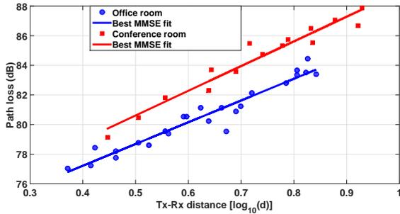
Fig. 5: Path loss model in the investigated office and conference rooms. In each case, the solid line is obtained with the MMSE estimator.
